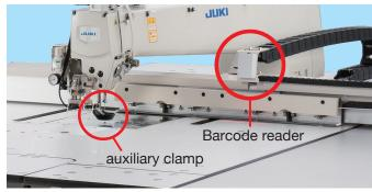
The barcode reader reads the barcode on the cassette clamp and automatically selects the corresponding sewing pattern.
