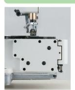
The longitudinal position of the feed is adjustable. As a result, uneven material feed and puckering that are likely to occur when sewing products made of elastic materials such as foundations are reduced. This means that the machine means that the machine promises imporved responsiveness to elastic materials.
