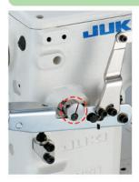
Elastic material or delicate material can be sewn with the presser foot kept slightly raised. This effectively helps reduce the degee of slippage, warpage and damage fo the material.
