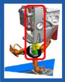
Optional attachment allows for the quick change over of presser foots for multiple processes. Presser foot holder will improve the productively and reduce down time for the most skilled operators.
