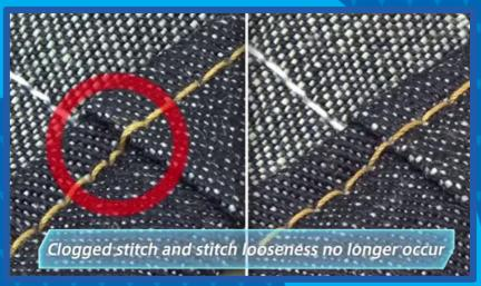
Stitch length, feed dog height and feed locus are all corrected automatically helping to elevate clogged stitches.
