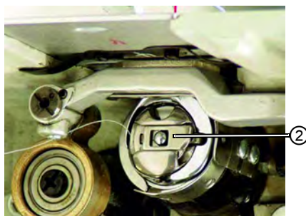
Figure 10: Replacing the hook thread bobbin
