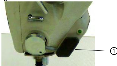
(1) - Pushbutton on the machine arm
