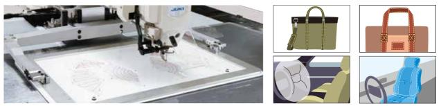
The sewing machine is used for many different applications where the machine takes advantage of its large sewing area, such as attaching handles to bags and pouches, attaching belts, sewing two or more small parts at a time,
