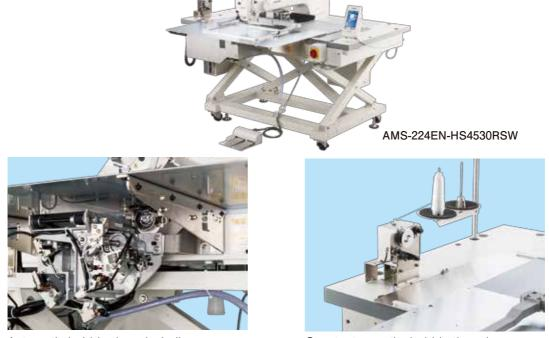
Automatic bobbin-thread winding and feeding unit
