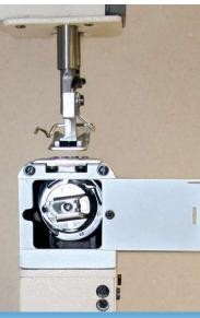
Machine is equipped with extra large diameter of hook.
